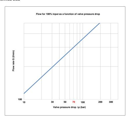
The diagram shows the maximum controlled flow rate according to the valve pressure drop between ports P & T
