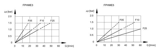
NOTE 2: The filter size has to be selected so that with the nominal flow rate the pressure drop is lower than 0.8 bar.
